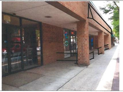
1.Install new section of awning on 12 & 20 East 4<sup>th</sup> St opening between piers. Match existing awning style of 8 East 4<sup>th</sup> Street.
